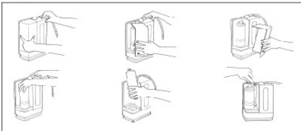
Cover latch>Gently opening cover>Cover detachment>Rotating filter>New filter foil removal>Filter life indicator reset
