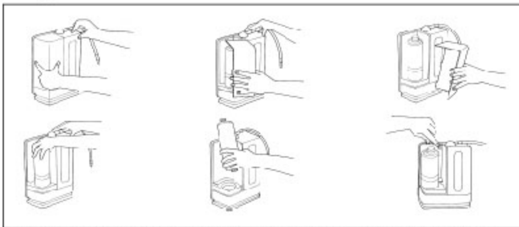
Cover latch>Gently opening cover>Cover detachment>Rotating filter>New filter foil removal>Filter lift indicator reset
