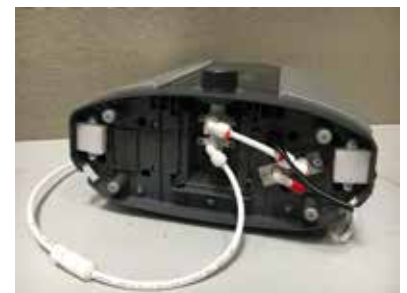
3. In-line Sediment Filter installed.
