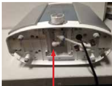
2. Install shortest part of tubing at Tap Water Inlet.
